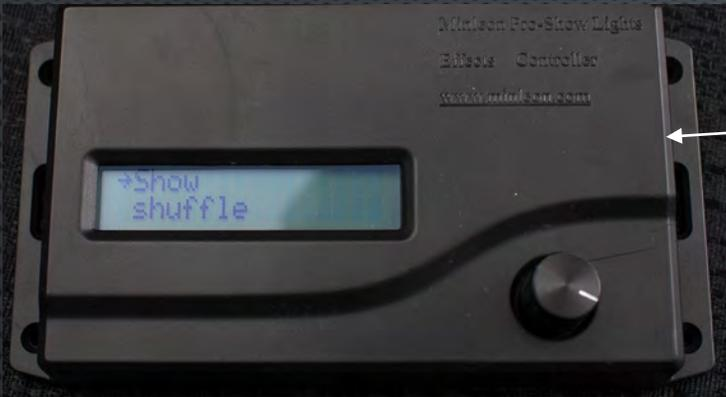
To date, custom sequence files from X-Lights & LightShow Pro can be exported to a .BIN file, and copied to an SD Card for playback on the NEC. Audio files in .WAV format can be triggered to synch with your sequence file.
